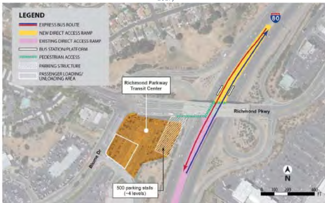
Figure 4: Proposed Ramp Improvements at Richmond Parkway Transit Center (West Contra Costa High Capacity Transit Study, 2017)
