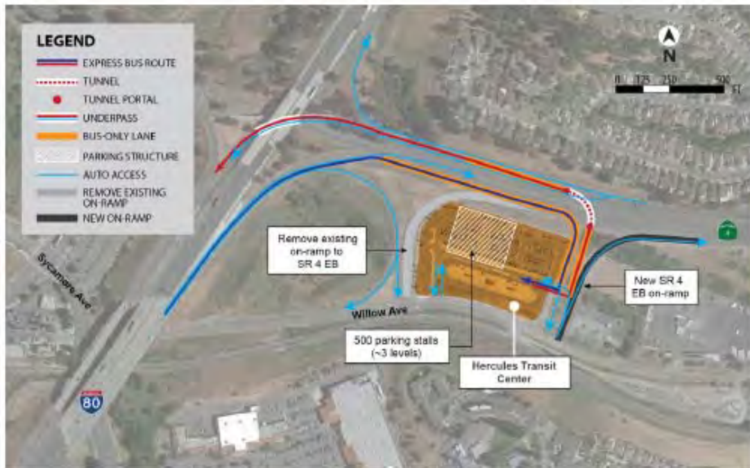
Figure 3: Proposed Ramp Improvements at Hercules Transit Center (West Contra Costa High Capacity Transit Study, 2017)
