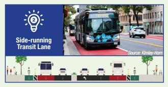
Side-Running Bus Lanes have stations that are placed on the side of the road and may include a bus island to allow bikes to pass behind the stop.
