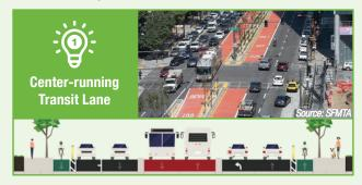
Center-Running Bus Lanes have stations that are placed in the median and accessed via crosswalks at existing or new signals.
