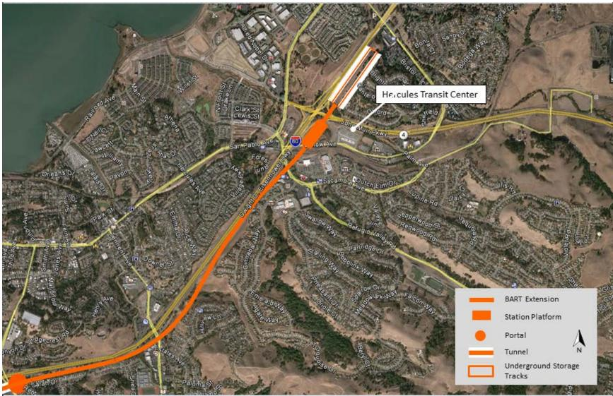
Figure 6-19: Hercules Terminus Station – Platform Option 4: East of I-80
