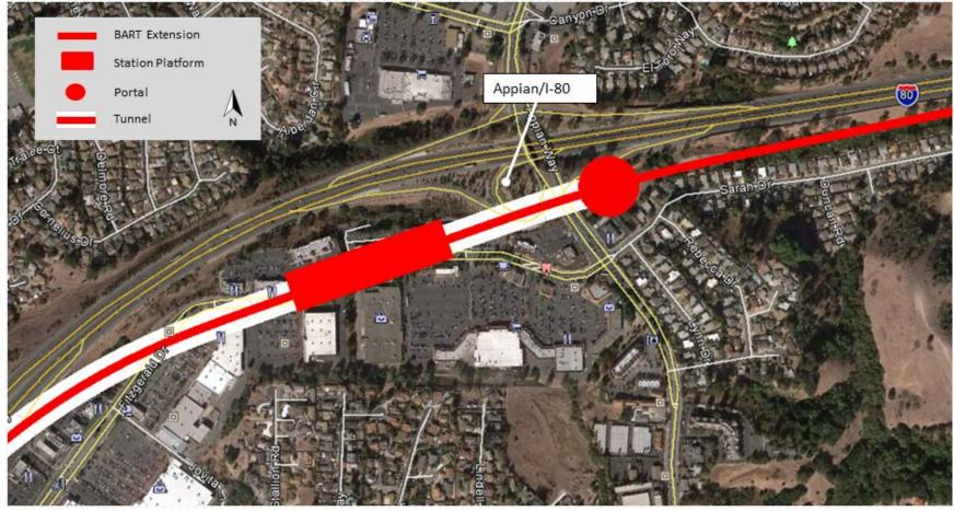
Figure 6-13: Refinement of Alternative 6: BART Extension – Richmond Parkway Alignment – Station Platform at Appian/I-80
