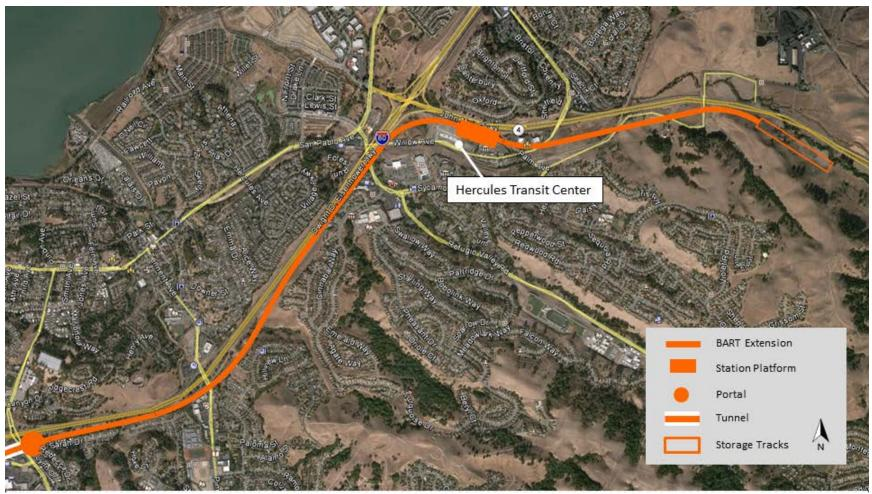
Figure 6-16: Hercules Terminus Station – Platform Option 1: Parallel to SR-4
