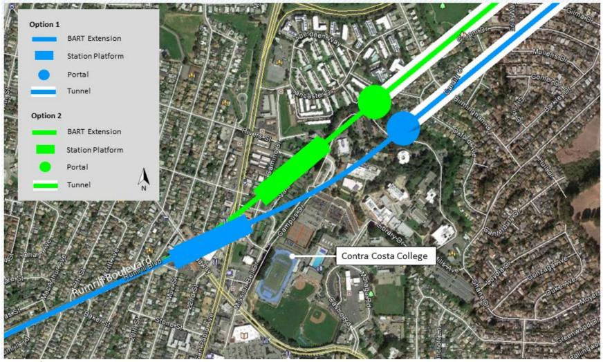
Figure 6-6: Refinement of Alternative 6: BART Extension – Rumrill Boulevard Alignment – Platform near Contra Costa College – Options 1 and 2
