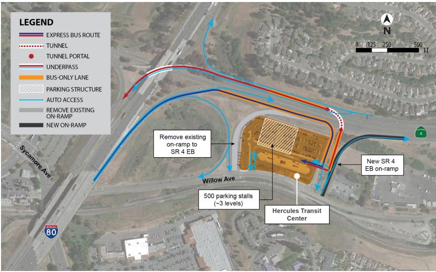
Figure 2-3: Refined Access to Hercules Transit Center – Tunnel and Underpass Option
